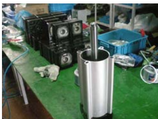
Assembling of the cylinder.
